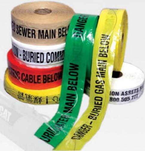
"GOLDEN" Brand Anti-Corrosive S.S wire Detectable Warning Tape is a coloured plastic detectable tape for detecting buried underground services. S.S. Wire detectable tape is manufactured using one or more stainless steel wires incorporated in sinusoidal pattern and encapsulated between two layers of low density lead free polyethylene film.
